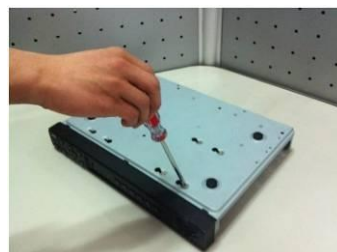
⑤ Fix the HDD firmly.
