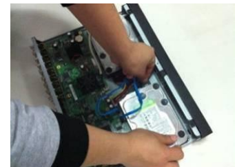
⑥ Connect the HDD cable and power cable.
