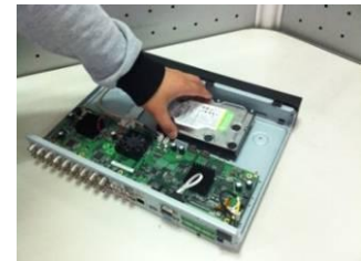
③ Place the HDD in accordance with the four holes in the bottom.
