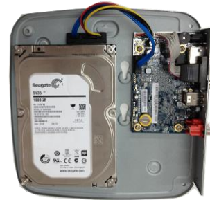
⑥ Connect the HDD cable and power cable.
