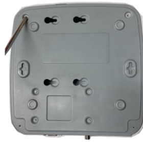
⑧ Secure the screws in the rear panel and the side panel.
