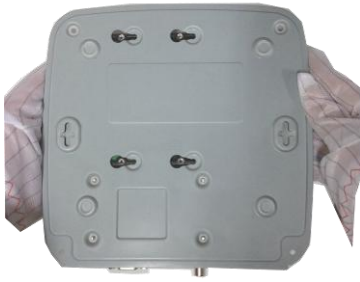
④ Turn the device upside down and then turn the screws in firmly.
