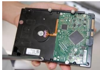
② Fix four screws in the HDD (Turn just three rounds).
