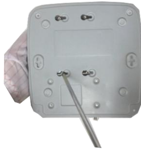
⑤ Fix the HDD firmly.
