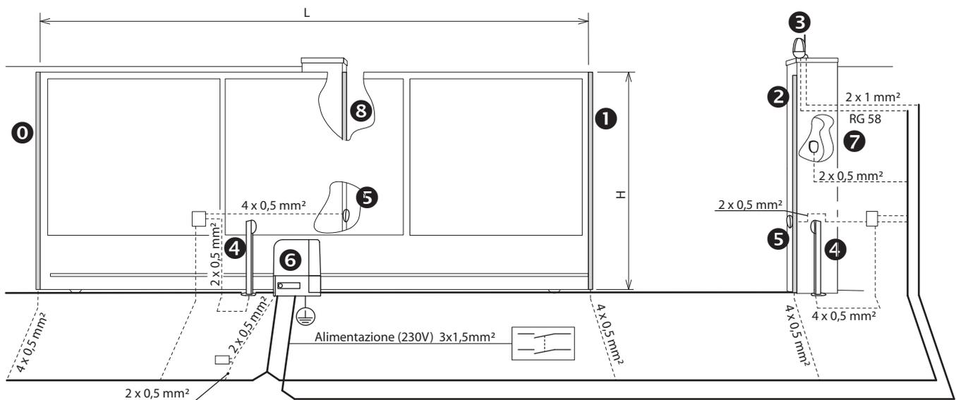
**COLLEGAMENTI ELETTRICI DEI SINGOLI COMPONENTI ESEGUITI CON LA CENTRALE DI COMANDO CHE PUO' ESSERE INCORPORATA NEL GRUPPO MOTORE O POSIZIONATA IN BOX ( 100G, 100GR, 100GG O 100A ) FISSATI AL MURO**
